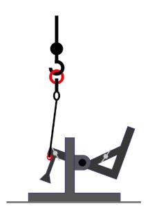
After successfully turning the wall section, the turning aid must be carefully turned back. This must only be done with the aid of the crane and never by hand!
