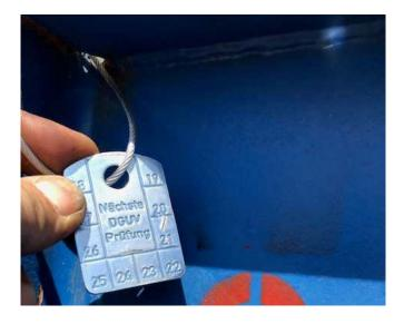
A valid DGUV inspection plate is located on the frame.
