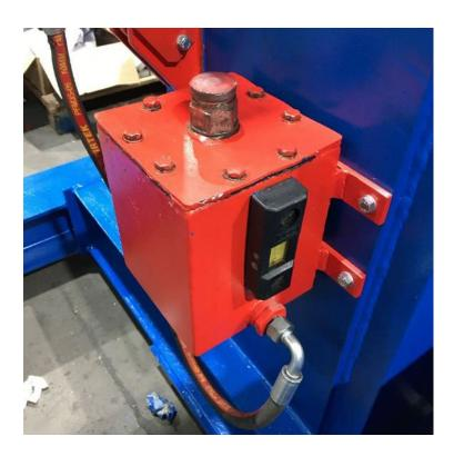
The hydraulic tank must always be filled to approx. 3/4.
